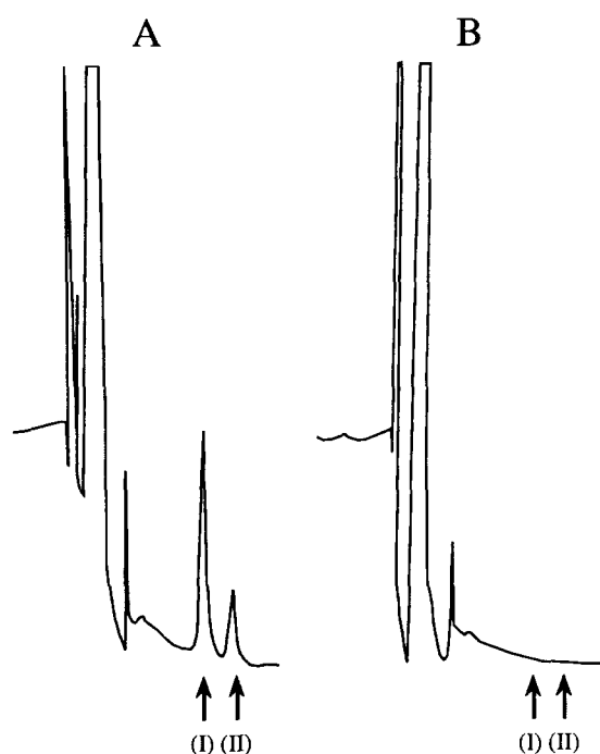
Figure 3 Chromatograms of (A) human urine containing 8.4 µg of ceftibuten (I) and 3.0 µg of ceftibuten-trans (II) per ml and (B) blank human urine.
